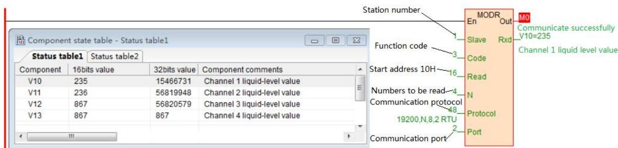
The host PLC reads the 4-channel liquid level values of S04AI by Modbus read instruction MODR, the start address is 10H (hexadecimal), that is, the decimal value is 16. When the communication is successful, M0 is ON, the liquid level values which are read back will be stored in V0-3, V0=235, indicating that the actual temperature of the first channel is 0.235m, the same as V3=867, indicating that the actual temperature of the fourth channel is 0.867m.
